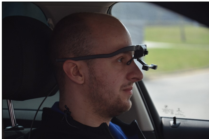
Obr. 29: Proband s eyetrackerem Dikablis Glasses 3 [77]
