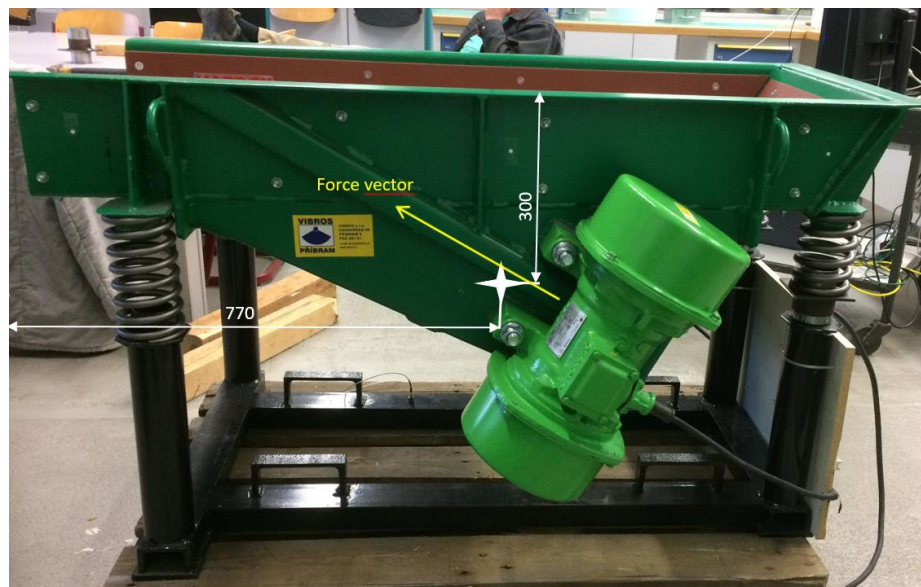
Figure 62: New centre of elasticity
