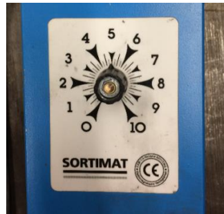
Figure 82: Operation controller of 2-mass linear vibratory conveyor on 50 % operation power
