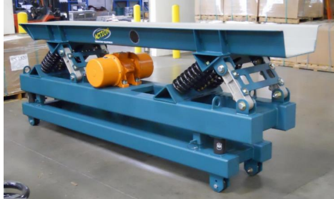
Figure 17: Vibratory conveyor with two masses of variant D
