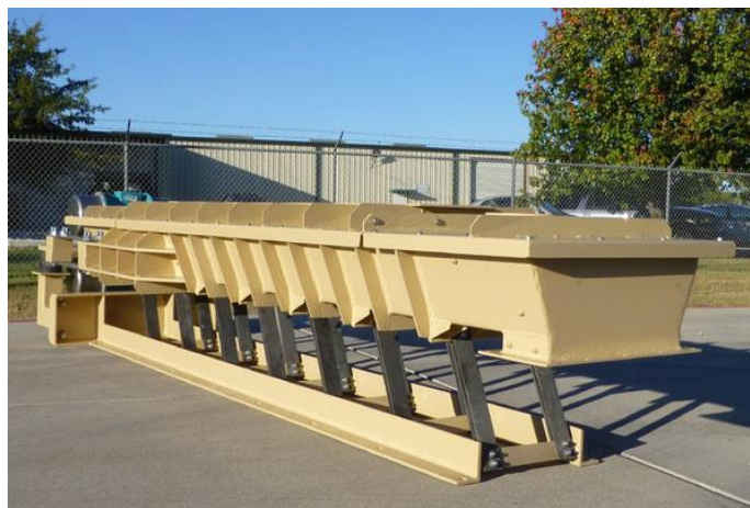
Figure 14: Guided linear vibratory conveyor of variant B with flat springs
