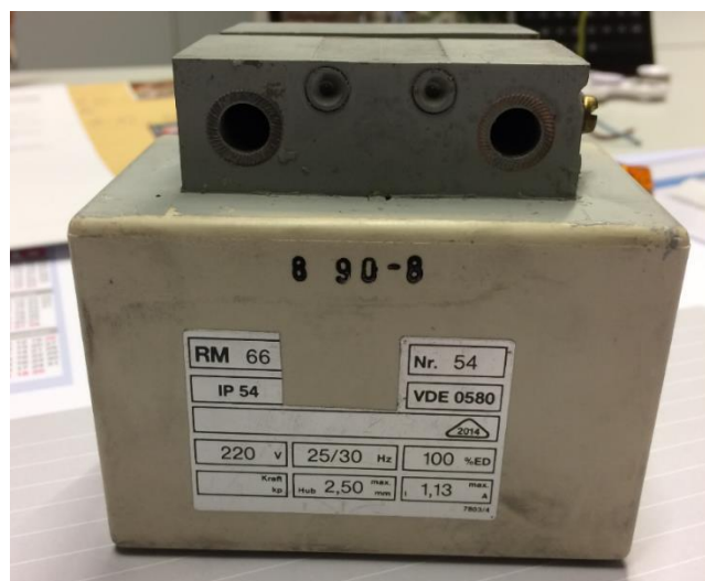
Figure 77: Electromagnetic exciter and its technical data
