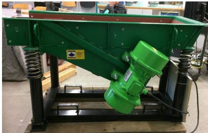
Figure 55: One-mass vibratory conveyor with modified springs
