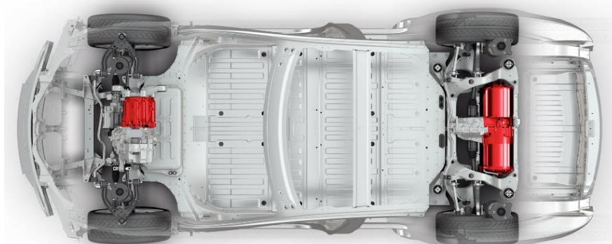
Obr. 2 Šasi a motory Tesla Model S [9]
