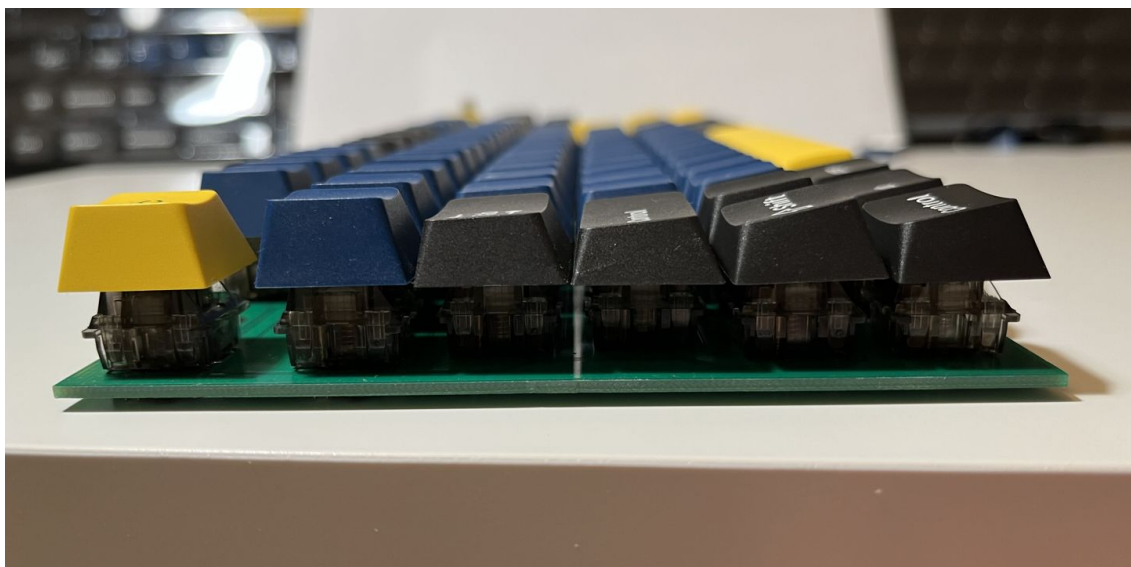
Fig. 26: The keycap profile.
