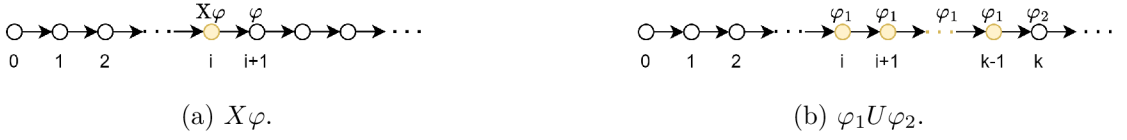
Figure 2.5: Visualization of next (a) and until (b) operators. The states for which the corresponding operator holds are colored.
