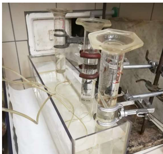
Figure 6.1. Inverted measuring cylinders with the collected gas after the production was stabilized
