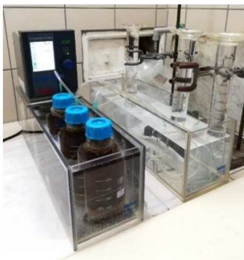
Figure 5.7. Reactors placed in optimal conditions and connected to the gas collecting system.
