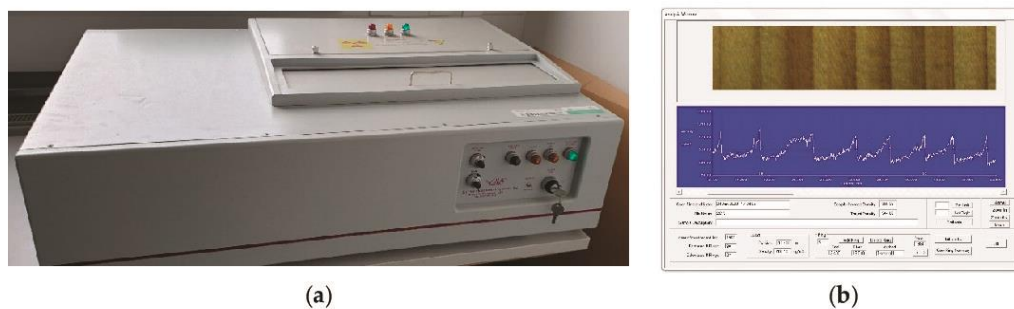
Figure 1. X-ray densitometer QTRS-01X Tree Ring Analyzer (a); wood density profile for one of the testing samples using QTRS-01X software (b).
