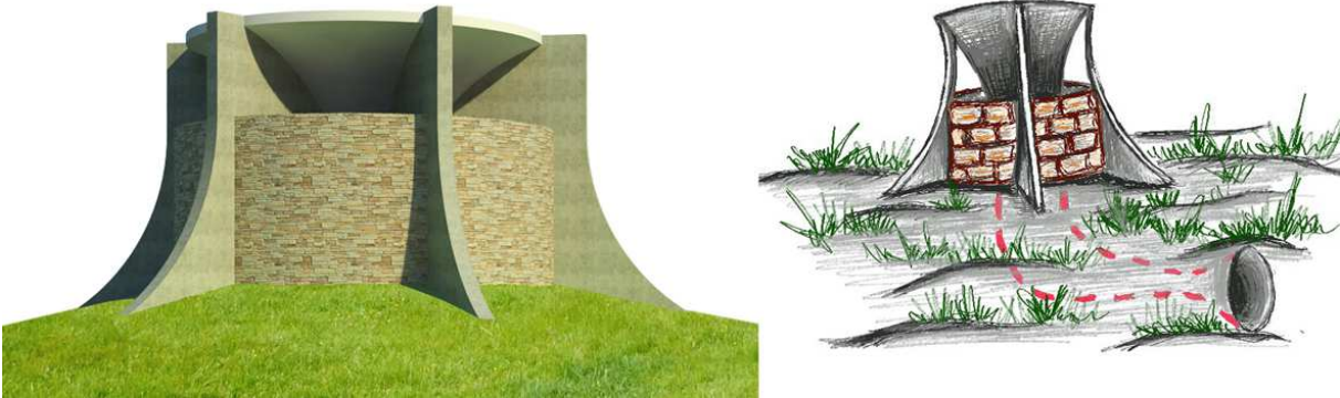
Fig. 5. Wind turbine presenting the structure partly hidden in the ground. The illustration shows intake built above the ground and the channel in the ground with exhaust revealing at the lower part of the hill.
