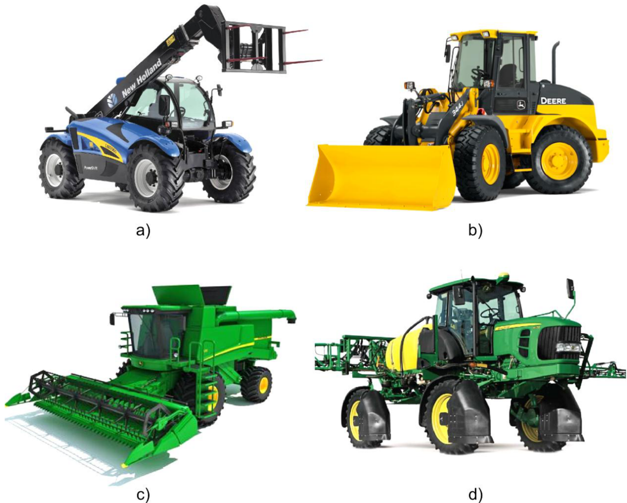
Fig. 6.2: Typical applications of HST. a) telehandler, b) wheel loader, c) combine harvester, d) sprayer.
