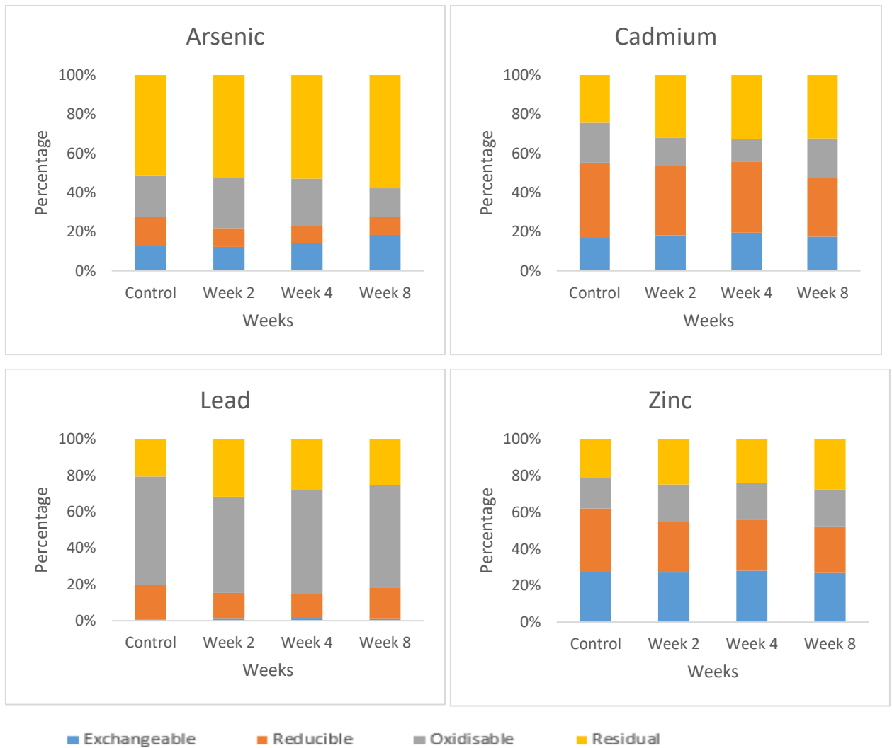
Fig.12. Evaluation of the fraction distribution of the soil sample amended with vermiculite.
