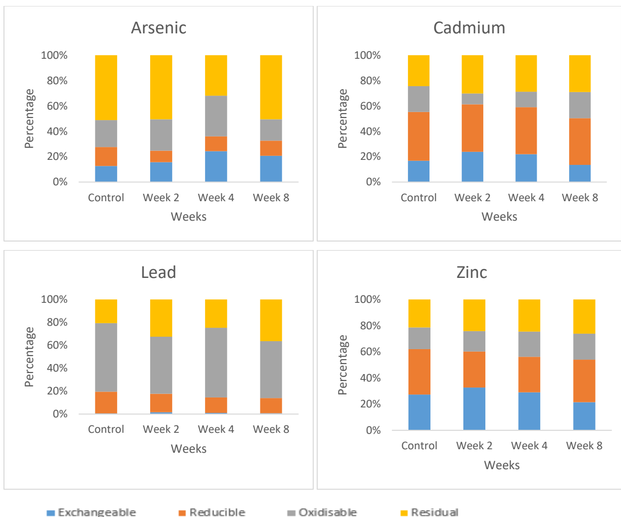
Fig. 10. Evaluation of the fraction distribution of the soil sample amended with kaolinite
