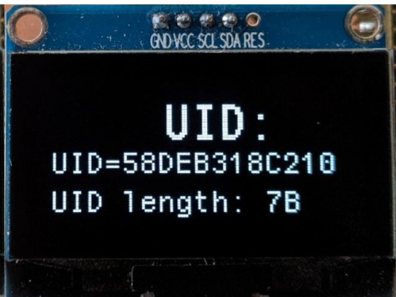
f) Transponder with 7B long UID
