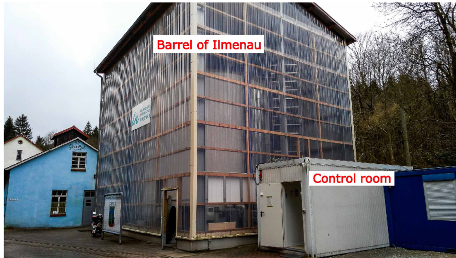
Fig. 2.1: Experimental facility Barrel of Ilmenau is a worldwide largest experiment for the study of highly turbulent convection in dry air. Diameter D = 7.15 m, height L can be adjusted up to 6.3 m).
