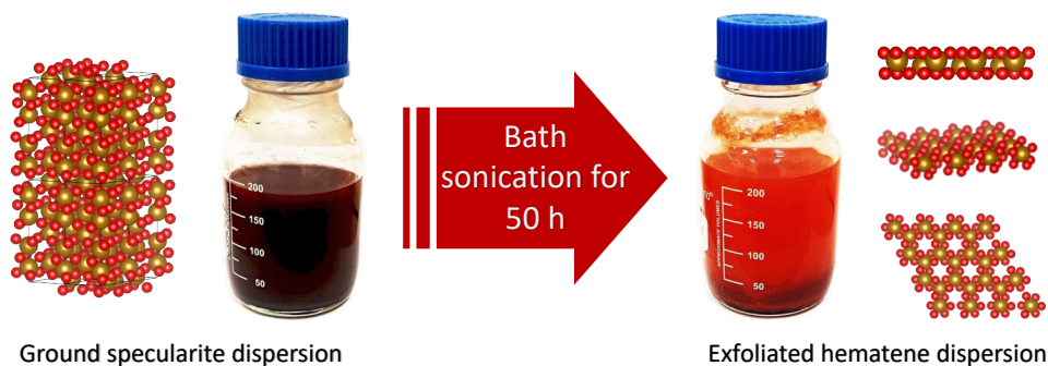
Figure 3.8: Scheme of exfoliation with photos of flasks with dispersions to illustrate the colour-change after sonochemical exfoliation.
