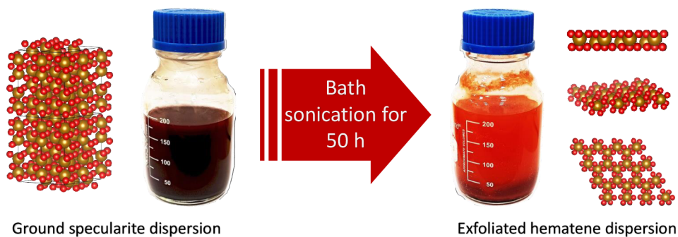
Figure 2.6: Scheme of exfoliation with photos of flasks with dispersions to illustrate the colour-change after sonochemical exfoliation.
