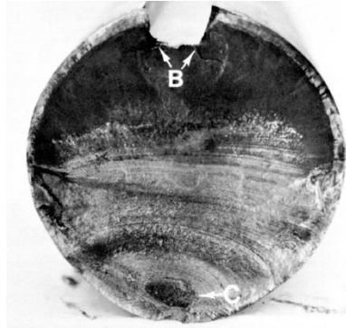
Figure 1.41: Fatigue fracture of a drive shaft. [8]
