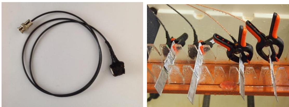
(a) AE sensors covered protection substance. (b) Installing the sensor on specimen.
