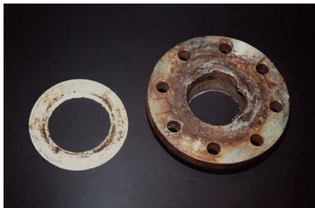
Figure 1.16: Crevice corrosion on steel flange exposed to a chloride medium. [93]
