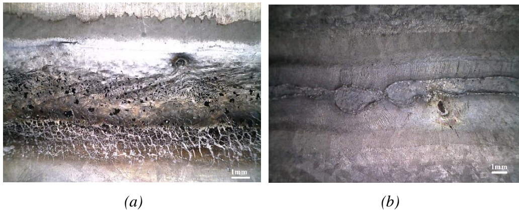
Figure 4.2: Micro-photographs of welding Al6065 to DX51D sheet at 73A welding current and 4.1m/min welding speed, (a) top surface of weldment, (b) back site of weldment.
