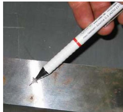
(a) Schematic diagram of Hus-Nielsen test. (b) Testing Hsu-Nielsen on test sample.
