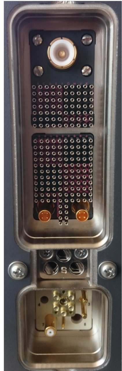
Fig. 3.1: ARINC 600 connector on LRU backplane
