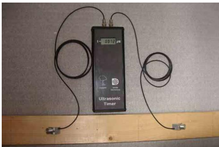
Obrázek 8: Fakopp Ultrasonic timer (2017)
