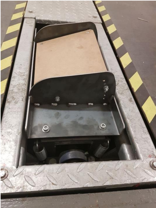
Fig. 4-2 Oscillating rig mounted on the tester.
