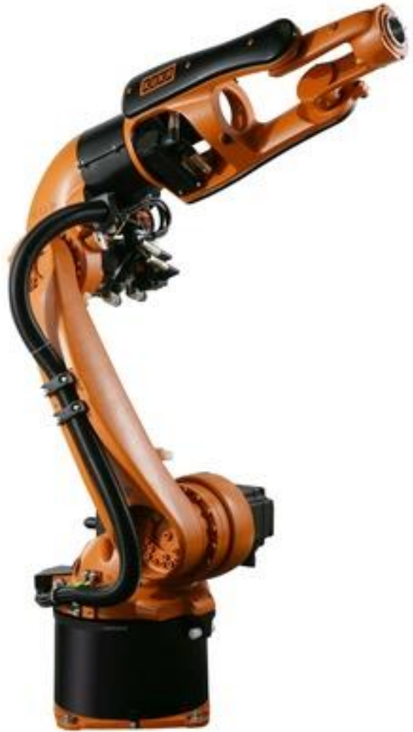
Obr. 19 Robot Kuka KR5arc HW [8]
