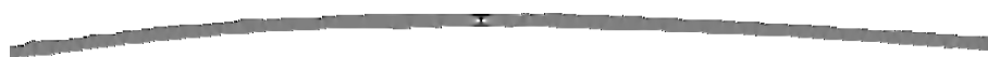
Fig. 6.23: Domain wall in the bent permalloy nanowire, simulation of \text{div}\vec{M} (magnetic charges) is shown in gray-scale for better comparison with MFM measurement, cell size 4 nm, damping 0.1. 'Black' part near the centre corresponds to the DW, other weaker contrast might be seen when diameter slightly changes and at the right end of the wire. Only crop of the nanowire with the DW is displayed.
