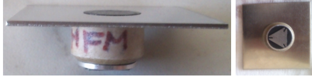
Fig. 6.7: Shielded sample holder for the Ntegra Prima microscope which consists of non-magnetic tubular ceramics with Al foil inside and 1mm thick Mu-metal plate and sticking tape for mounting the sample. The height of the holder is approximately 1 cm.
