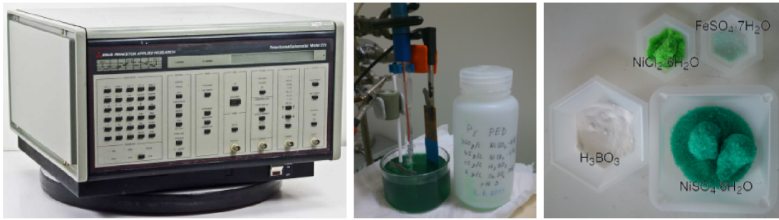
Fig. 5.2: Electrochemical deposition of nanowires. From the left: potentiostat (instrument for electrochemical experiments), deposition cell with electrodes and salts used for the electrolyte preparation.
