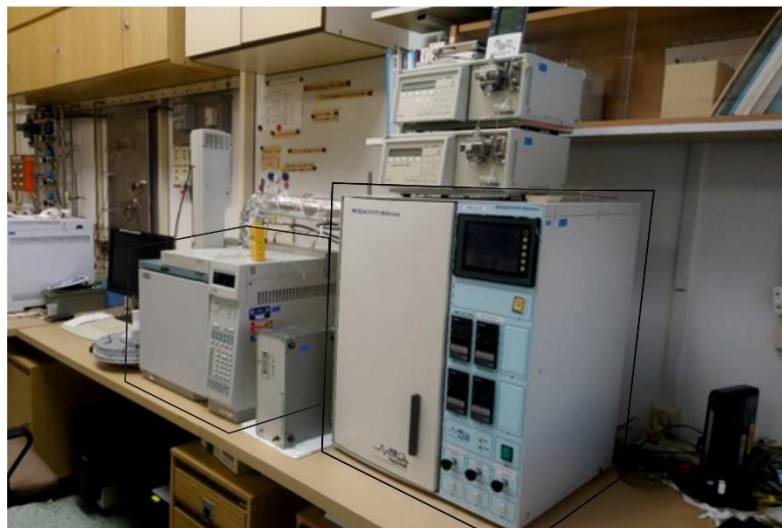
Figure 8. Microactivity Reactor System PID (on the right) with Agilent Gas Chromatograph (left). Both of the instruments are outlined.
