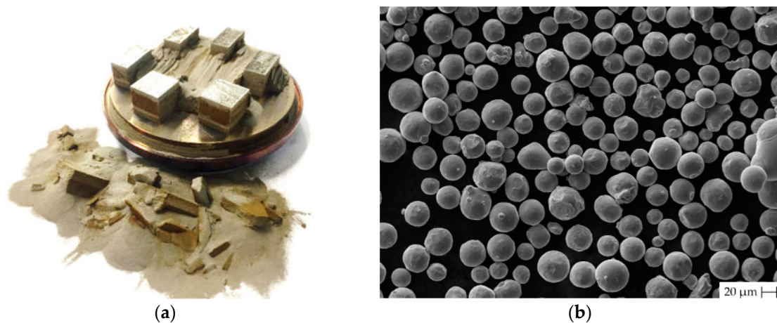
Figure 8. The powder used in heating unit preheated to the 550 °C (a) Build job made with 550 °C; (b) SEM microscopy photo of the powder used with 550 °C.
