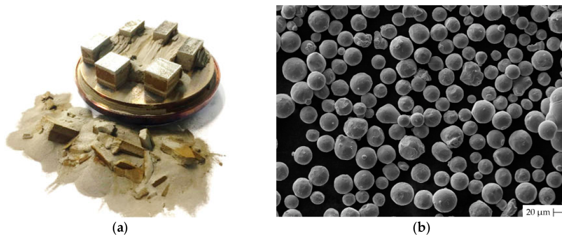
Figure 8. The powder used in heating unit preheated to the 550 °C (a) Build job made with 550 °C; (b) SEM microscopy photo of the powder used with 550 °C.
