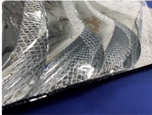
Fig. 4.2: Example of expanded MLI [22]
