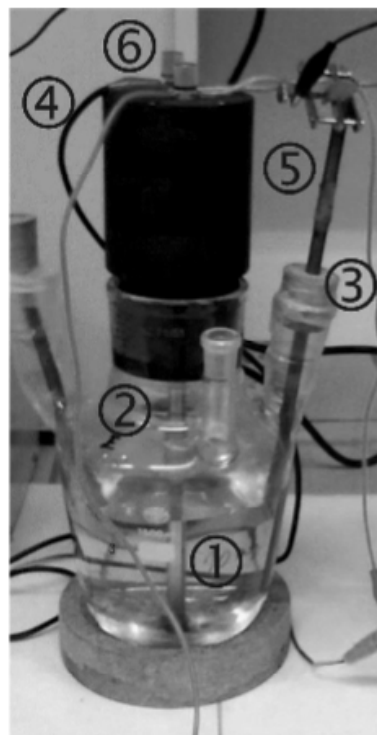
Fig. 1 Experimental apparatus: (1) HCH-spiked deionized water, (2) glass reactor, (3) rubber caps, (4) power lines to supply, (5) iron electrodes, (6) stirrer
