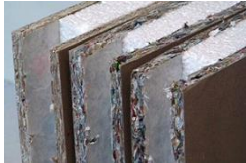
Figure 16: Construction boards made of recycled LPB
