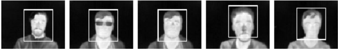
Figure 17 Some examples of face detection in different conditions using Chamfer Matching (Own Source)
