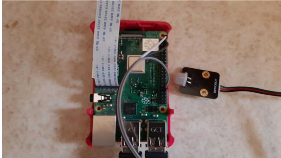
Figure 4 Raspberry Pi and peripherals final setup image (Own Source)
