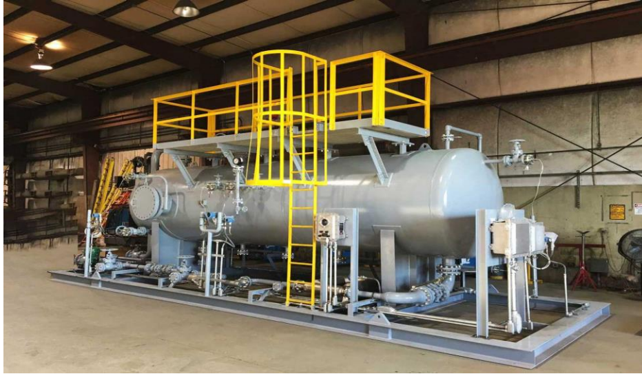
Figure 3 3-Phase Separator (TechFab, 2022)
