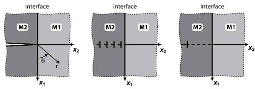
Fig. 4 Semi-infinite crack terminating perpendicular to the interface of two anisotropic materials.
