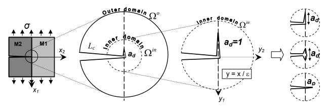
Fig. 7 Outer and Inner domain used in the matched asymptotic analysis (in case of the singly deflected crack) - zoomed-in view of crack neighbourhood perturbed by a small crack extension.
