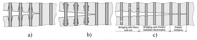
Fig. 3 Interface fibre/matrix: a) decohesion of fibre in matrix; b) frictional constraint fibre/matrix; c) characteristic bridging areas and corresponding types of constraints fibre/matrix.
