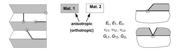
Fig. 1. Different types of the general stress concentrators – crack terminating at the interface of two dissimilar materials, interfacial crack, notch and V-notch and a general multimaterial wedge.
