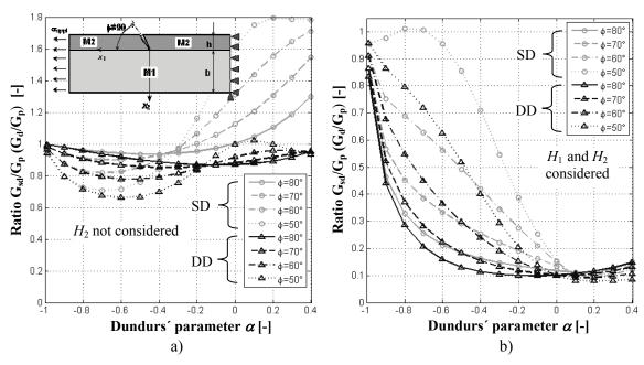
Fig. 9 Ratios  $G_{sd}/G_p$  and  $G_d/G_p$  as a function of Dundurs' parameters  $\alpha$  for several values of the crack inclination angle  $\phi$  (the characteristic crack extension length  $\varepsilon=1/100$ ) a) the case when the second singular term is not considered  $(H_2=0)$ ; b) both  $H_1$  and  $H_2$  singular terms are considered.
