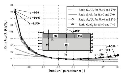
Fig. 8 The ratio of  $G_{sd}/G_p$  ( $G_d/G_p$ ) as a function of Dundurs' parameter  $\alpha$  for several values of the characteristic crack extension size  $\varepsilon$ . (sd-single deflection, d-double deflection, p-penetration).
