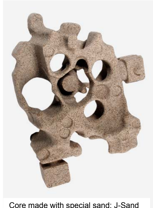
Core made with special sand: J-Sand
