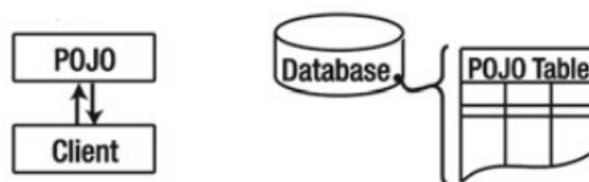
Figure 1.13: Detached objects exist in the database but are not maintained by Hibernate. Taken from [36].
