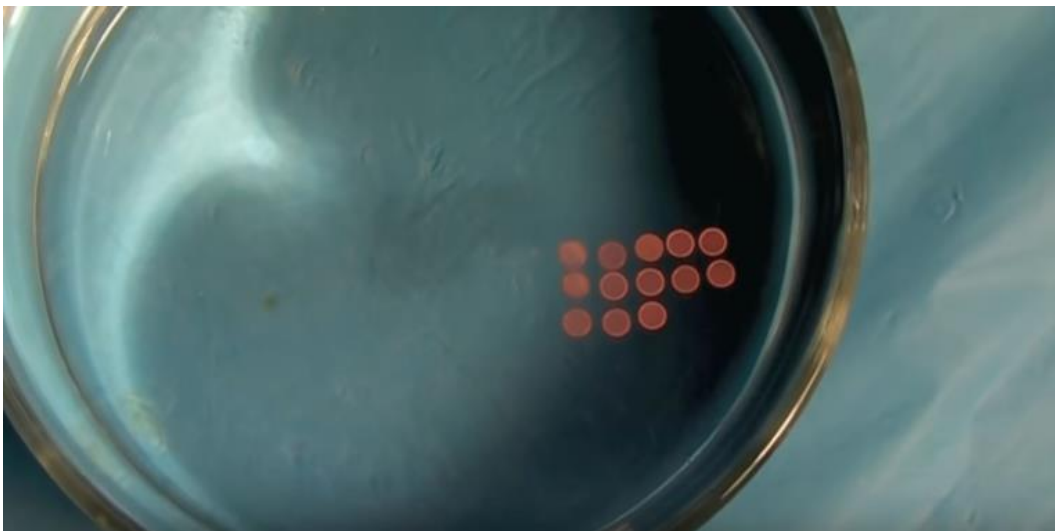
Figure 12: TEM grids on a formvar film floating on distilled water.
