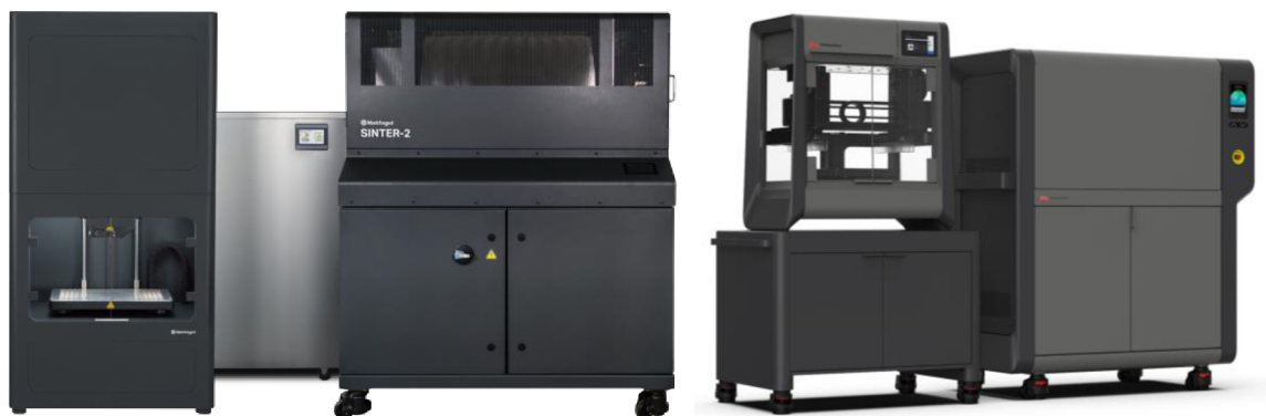
Obr. 2-12 Markforged Metal X (vlevo) vs Studio System 2 (vpravo) [31] [18]
