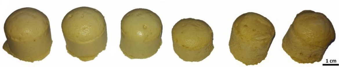
Fig. 67 CaP/PU foams having \frac{ha}{polyol} \text{ ratio} = 1 and I_{NCO} = 105 (water content increasing from 0 wt.% (left) to 5 wt% /(right) of polyol)
