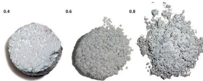
Fig. 78 Overview of scaffolds containing 4% H 2 O: (a) ha/pu = 0.4, (b) ha/pu = 0.6, (c) ha/pu = 0.8
