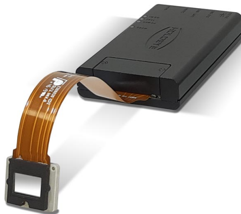
Figure 3.6: PLUTO-2.1 LCOS Spatial Light Modulator.
