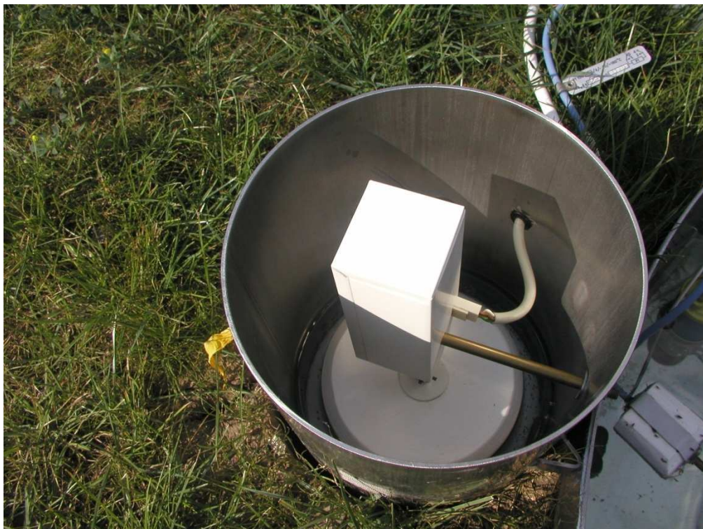
Figure 3. Optical sensor of EWM pan
