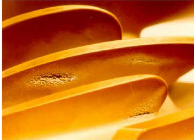
Figure 2. Cavitation erosion on pump impeller [17]
