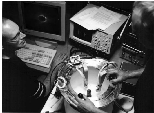
Figure 2-5: Experimental prototype of the 2D USCT system in Forschungszentrum Karlsruhe. The white tank is filled with water as a coupling medium for the examined object. Two ultrasonic probes are mounted on rotated rings to simulate all emitter and receiver positions. (Taken from [65])
