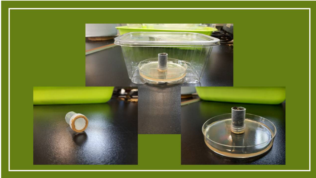
Figure 6: Experimental design of the soil column experiment. Pictured here: soil column in plastic box, column on its own, soil filled column on Petri dish
