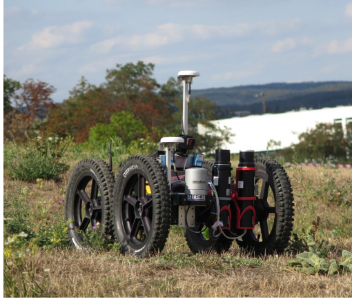
Figure C.10: The Orpheus-X4 UGV equipped with a GNSS receiver and a pair of NaI(Tl) radiation detectors.
