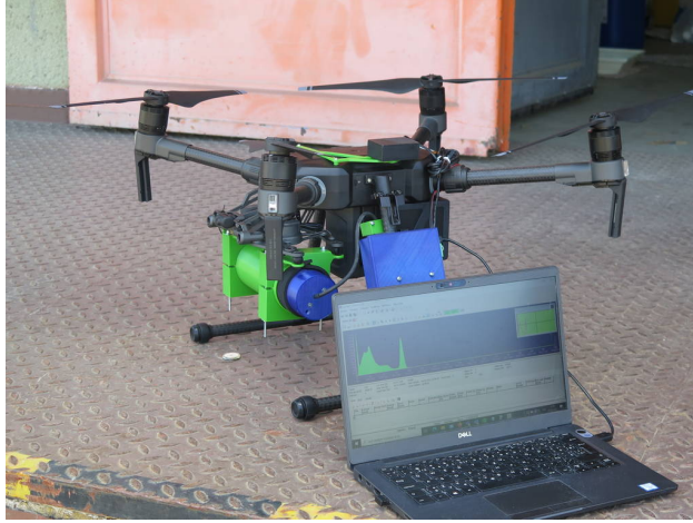
Figure D.4: The unmanned aircraft with a radiation detection system, and the live spectrum visualization.
