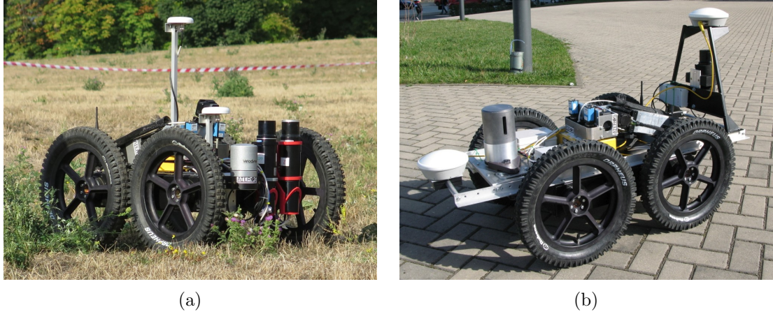
Figure 3.1: The UGV Orpheus-X4 equipped with a pair of scintillation detectors (a) and a collimator-based detection system (b).
