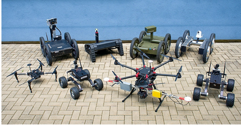
Figure C.1: The four-wheel Orpheus robot family and other platforms of the heterogeneous reconnaissance mobile robot system ATEROS.
