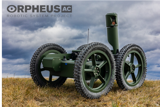
Figure 4.2: The decontaminable terrestrial robot Orpheus-AC3.
