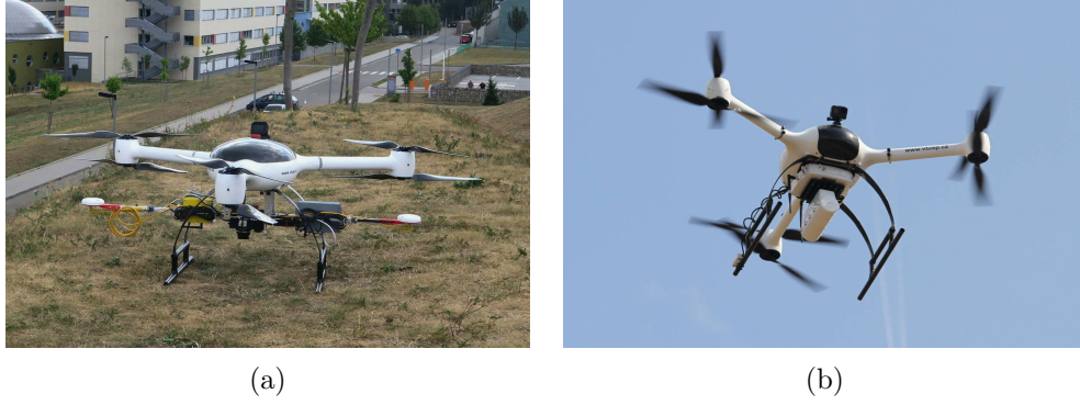
Figure C.9: The BRUS UAS configured for the experiment: with a multi-sensor system to perform the photogrammetry (a), and carrying a gamma radiation detection setup (b).
