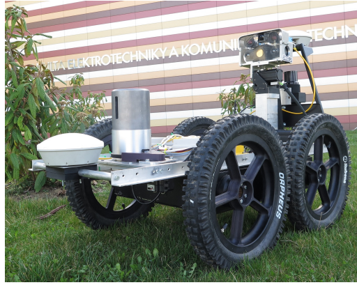
Figure B.2: The Orpheus-X4 carrying the detection head.
