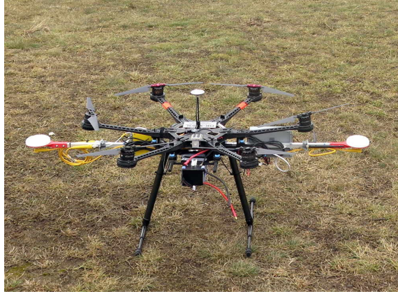
Figure A.2: The DJI S800 UAV equipped with the multi-sensor system for direct georeferencing.
