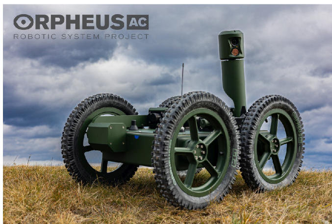
Figure 4.2: The decontaminable terrestrial robot Orpheus-AC3.
