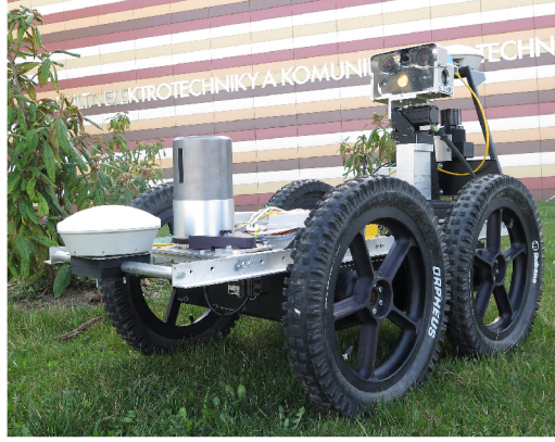
Figure B.2: The Orpheus-X4 carrying the detection head.
