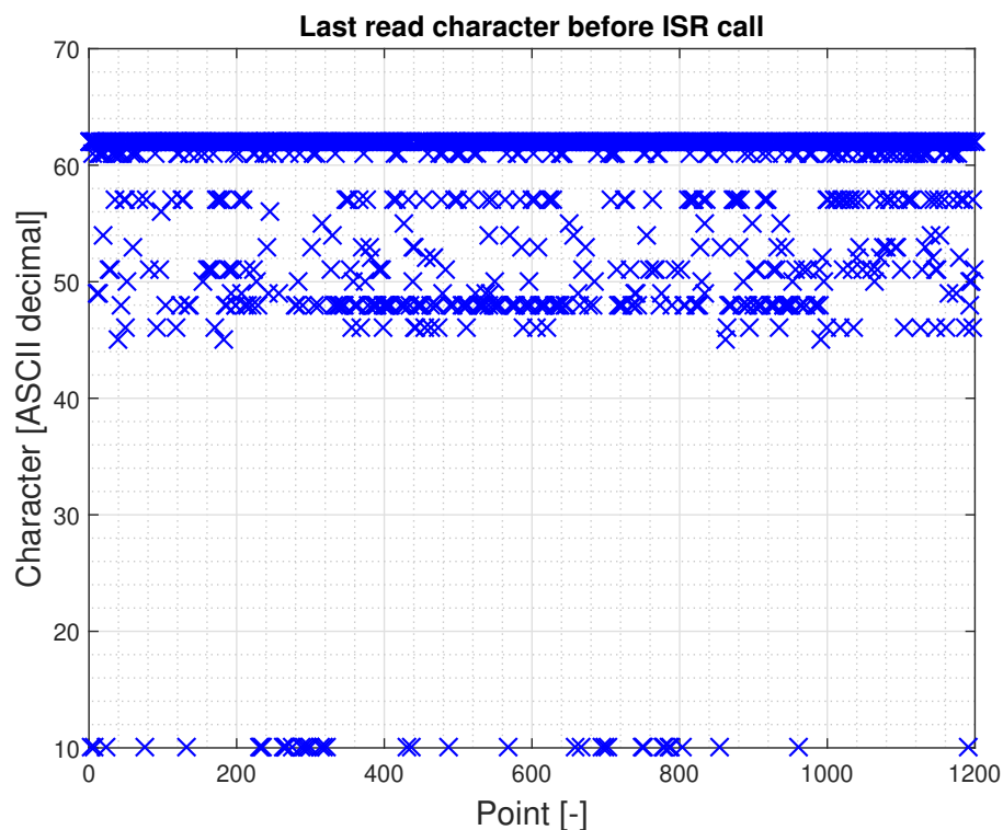
Fig. 5.11: Testing interrupt-driven time-stamping on UART.
