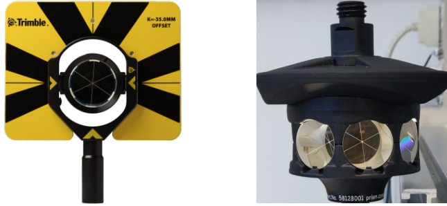
Fig. 2.5: An example of a circular (left) and 360 (right) prism. Left: taken from [19].
