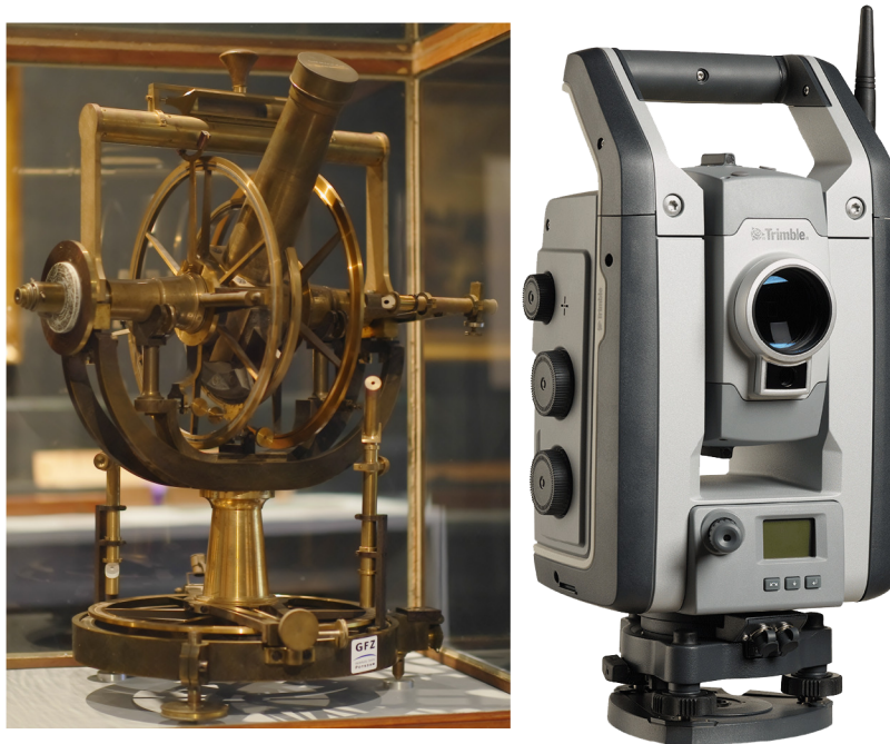
Fig. 2.1: A visual comparison of an old and modern theodolite. Left: taken from [3], Right: taken from [4].
