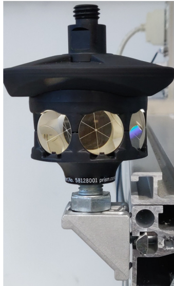
Fig. 5.14: Prism placement for horizontal rotation tests.
