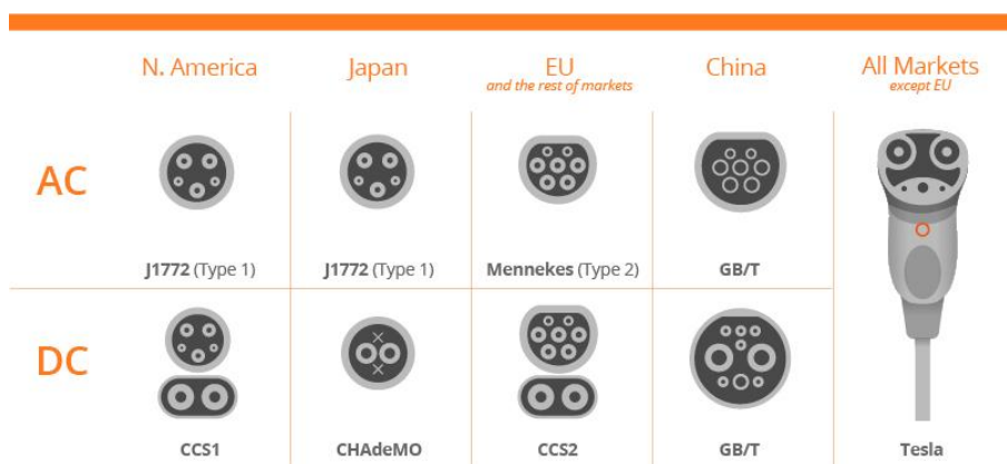
Figure 9 Charging connector types Source: https://evcharging.enelx.com/eu/about/news/blog/552-ev-charging-connector-types
