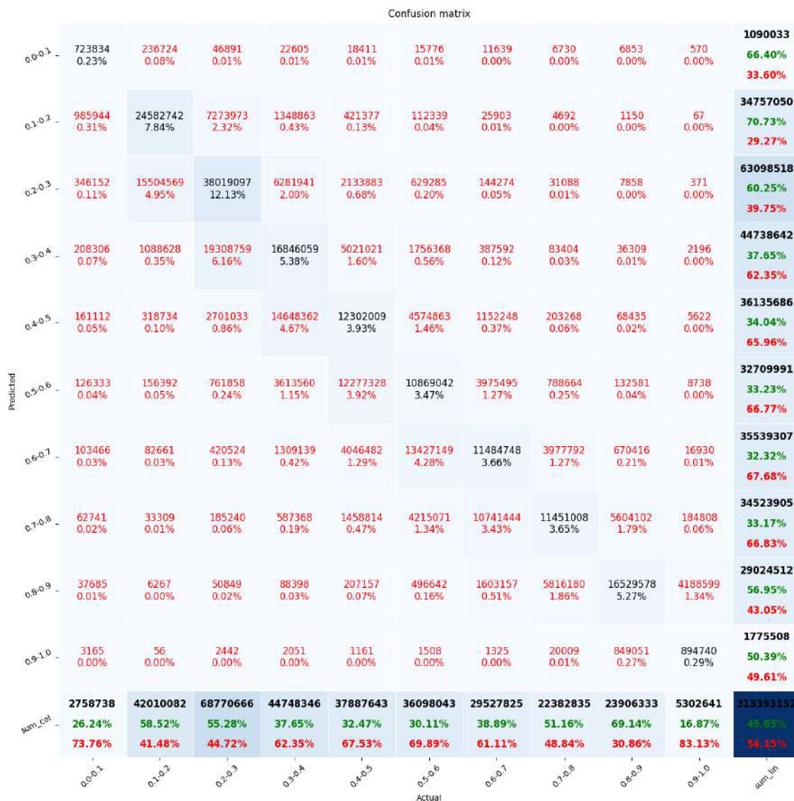
Figure 6.14: Confusion matrix for model 3. Compares predicted pixels with present NDVI for test data of the All dataset. Provides more insights into pixel distribution. The axis shows a value range between 0 and 1 with steps equal to 0.1. At the edge, aggregated data are shown. Aggregated values show the percentage of how many pixels were recognized correctly and incorrectly per row/column. The black and red colour in the graph core represents correctly and incorrectly assigned values. Unlike the percentages on edge, the core of the graph shows overall percentages.
