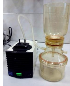
Fig. 3-11 Vacuum sorption apparatus: 1-funnel; 2-sorbent; 3-sorbent supporting unit; 4-vacuum pressure port; 5-vacuum flask.
