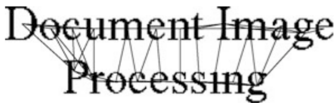
Figure 4.13: An example of connected components using k -nearest neighbor algorithm (the bottom-up strategy) [Kise, 2014].
