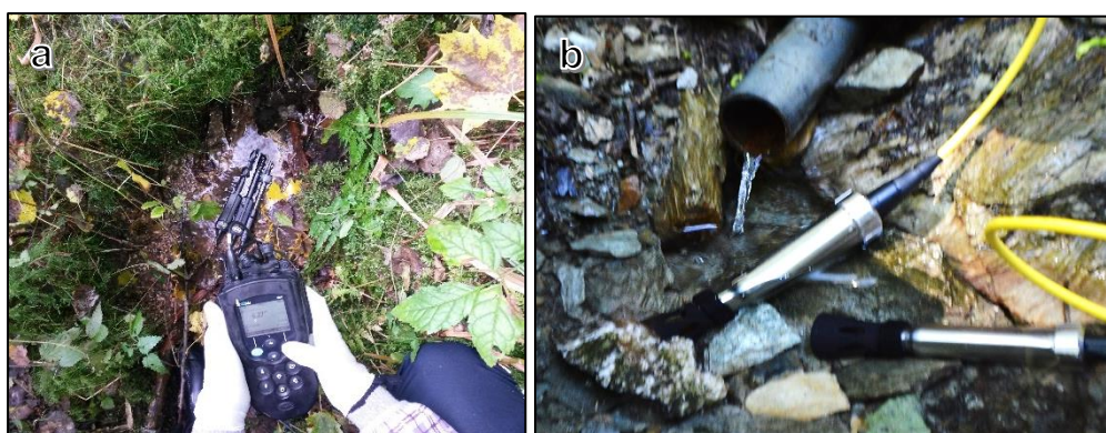
Fig. 20 Physico – chemical water parameters (a and b measurement of water parameters using the handheld digital analyzer for pH, temperature, conductivity and DO)
