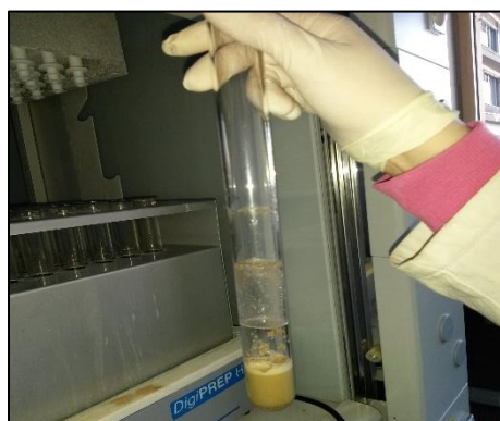
Fig. 26 Reduction of volume of the residue between 2 – 3 mL
